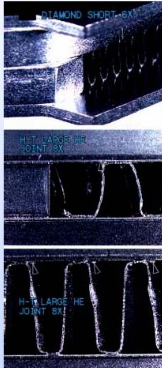
Three macrographs of an Inconel 625/MBF-51 brazed heat exchanger depicting a general view and magnified views of a narrow and a wide passages.
