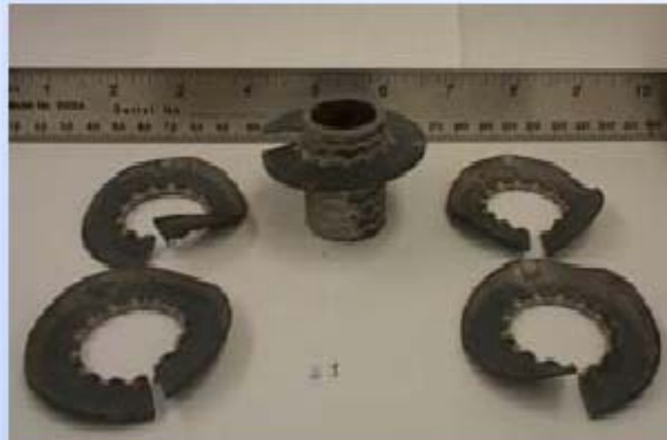
Testing of low-carbon steel pipe/fin parts brazed with BNi-2 (MBF-20 METGLAS® Foil) narrow (~3 mm) foil strip. (a) Tested part; (b) Instron setting during loading; (c) Parts after failure
